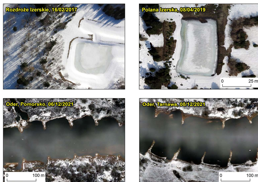
Figure 21. Fragment of single aerial image taken in central projection by a UAV over Rozdroże Izerskie in southwest Poland showing two interconnected frozen reservoirs ( top left ), fragment of the SfM-based orthophotomap of Polana Izerska in southwest Poland centered on a frozen reservoir ( top right ), fragments of the SfM-based orthophotomaps of the Oder River in west Poland in Pomorsko ( bottom left ) and Tarnawa ( bottom right ) showing an unfrozen river channel (source: Department of Geoinformatics and Cartography, University of Wrocław).
