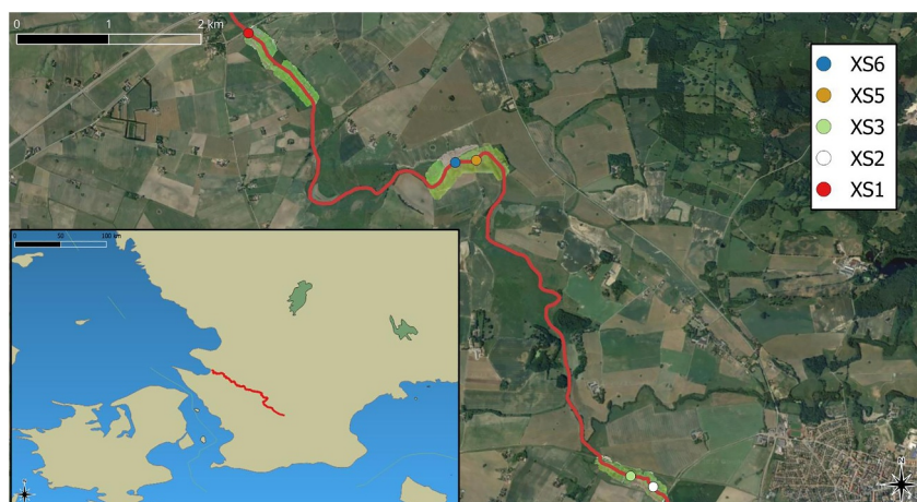
Figure 4. Map showing the measured locations in Rönne River in Sweden (source for the inset map is from Natural Earth Data ). Selected five cross-sections measured by the UAS-borne RSS-2-300W Doppler radar were shown in solid circles. Both red lines represent the river survey centerline.
