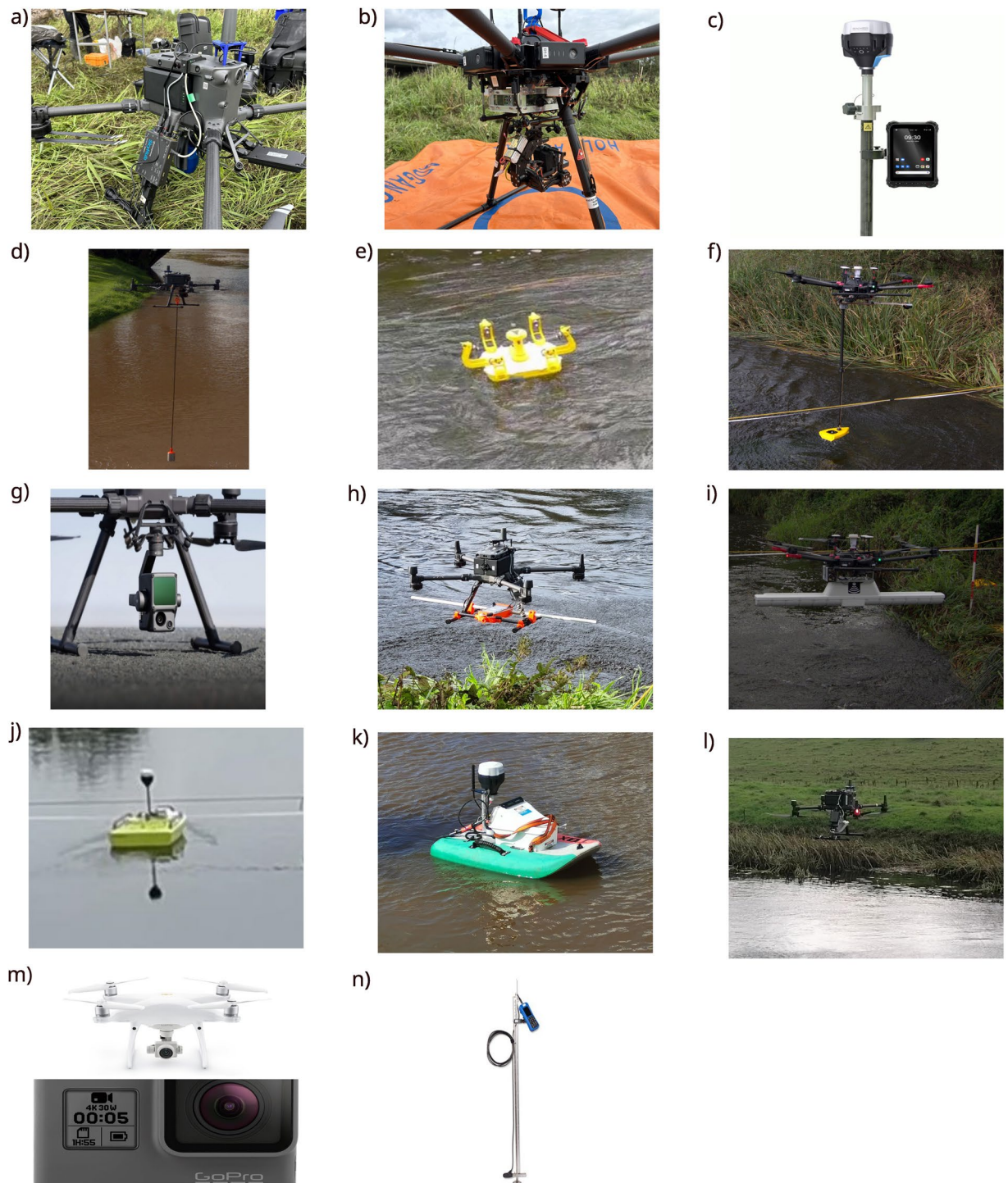
Fig. 4 (a–c), (g,m), and (n) show M300_LX80, M600_IWR1443, EMLID REACH RS2+, M300_Zenmuse L1 (integrating a Livox Lidar module and a camera), DJI Phantom 4 Pro (upper) and GoPro Hero 5 (down), and OTT MF Pro, respectively. (d–f) and (h–l) show the measurement processes of M300_ECT400s, Hydrohex_ECT400, M600_DeeperSmartSonarCHIRPplus, M300_Zond Aero LF, M600_Gekko 80, Boat_Teledyne RiverPro 1200, Boat_SonTek RS5, and M300_RSS300, respectively.
